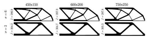
Figure 4: We demonstrate the mesh-independence of our method by visualizing density fields at different resolutions for a set of fixed  $\sigma$  values.
