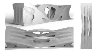
Figure 9: Bridge  $\sigma = 2.5$  in 320x160x80 trained for 3500 iterations. The design is mirrored along X and Z axes for visualization.
