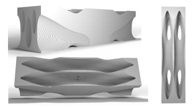
Figure 8: Bridge  $\sigma = 1$  in 320x160x80 trained for 3500 iterations. The design is mirrored along X and Z axes for visualization.
